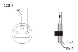
For installations where the DMX cable has to run a long distance or is in an electrically noisy environment, such as in a discotheque, it is recommended to use a DMX terminator. This helps in preventing corruption of the digital control signal by electrical noise. The DMX terminator is simply an XLR plug with a 120  $\Omega$  resistor connected between pins 2 and 3,which is then plugged into the output XLR socket of the last fixture in the chain. Please see illustrations below.
